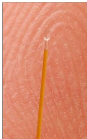
Photo shows a M260 pressure sensor of 260µm outer diameter on a finger
