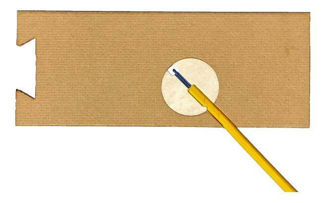
You should install the sensor in a 2,5mm thick spacer or more. You could stack some spacers.
