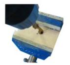
Drill a10 mm hole using mark 2 as the center.
