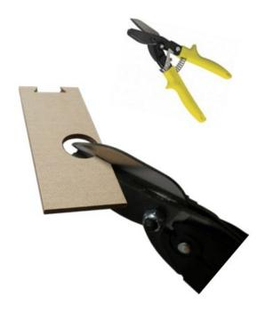
Take care that the cable slot cross the center of the hole, if the cable slot is offset from the center of the hole it could stress the fiber optic cable
