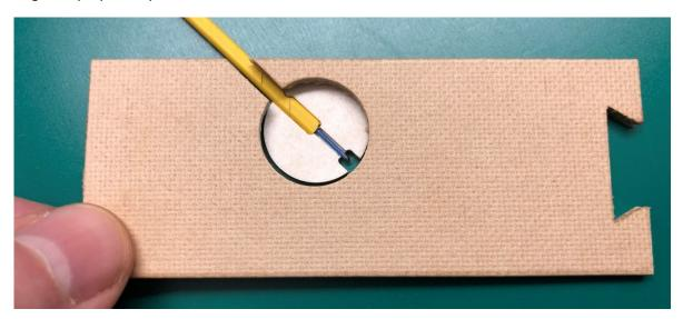
Press down the prepared spacer on the sensors and disk:
