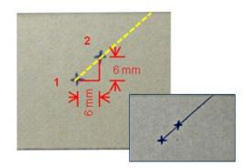
Draw a line that joins both marks and extend it to the edge. This becomes the position of the cable slot.
