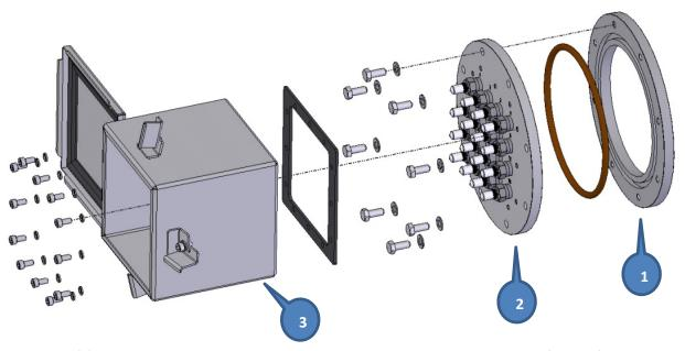
The EasyRing (1) is a carbon steel circular ring that can be welded to the tank wall to interface perfectly with the EasyPlate. Its Viton O-ring ensures that no leak is possible between the ring and the plate.
