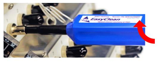
**Step 4:** Push the outer body a second time to clean the connector face
