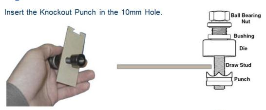
Using a ratchet a wrench or a drill, rotate the knockout punch nut, while holding the spacer, until the punch goes through.
